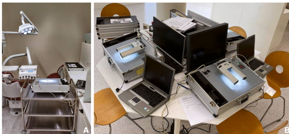
Figure 2. Experimental design. A, KaVoLUX 540 LED (LK) light source with adjusted light on Toothguide Training Box (TTB). B, D55 daylight lamp on Toothguide Training Box with associated laptop for data collection.
