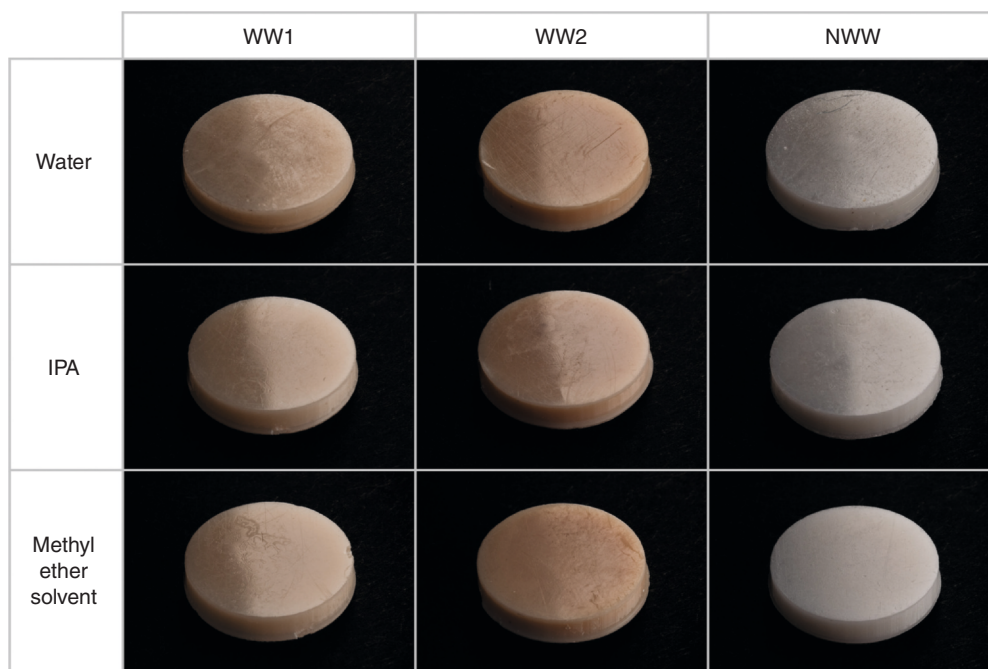
Figure 2. Representative images of specimens from each material-post-processing cleaning solution pair.
