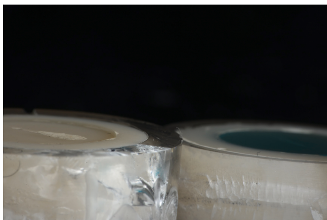
Figure 7. Macro images demonstrating material wear. Captured using a macro lens and auxiliary lens. Original magnification not precisely determined. A, PMA. B, PRT.
