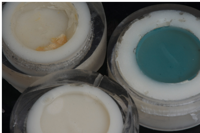
Figure 6. Macro images demonstrating material wear. Captured using a macro lens and auxiliary lens. Original magnification not precisely determined. A, PMA. B, MMA. C, PRT.
