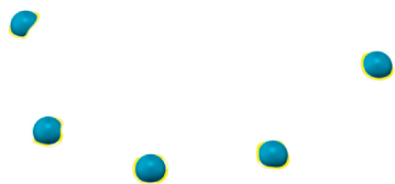
Figure 6. With predefined cutting surfaces (yellow) trimmed scan surface resulting in precision ball sections only relevant for evaluation (turquoise).
