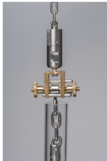
Figure 1. Bonded specimen in universal testing machine.
