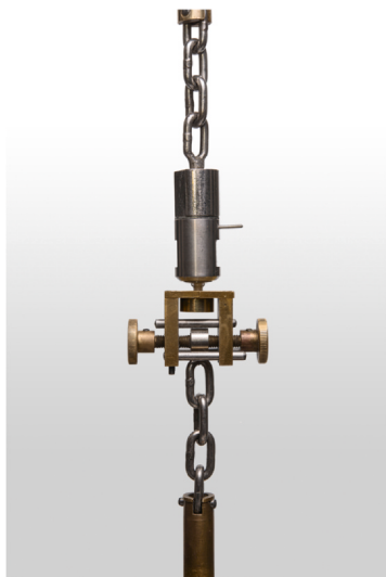
Figure 2. Bonded specimen in universal testing machine.
