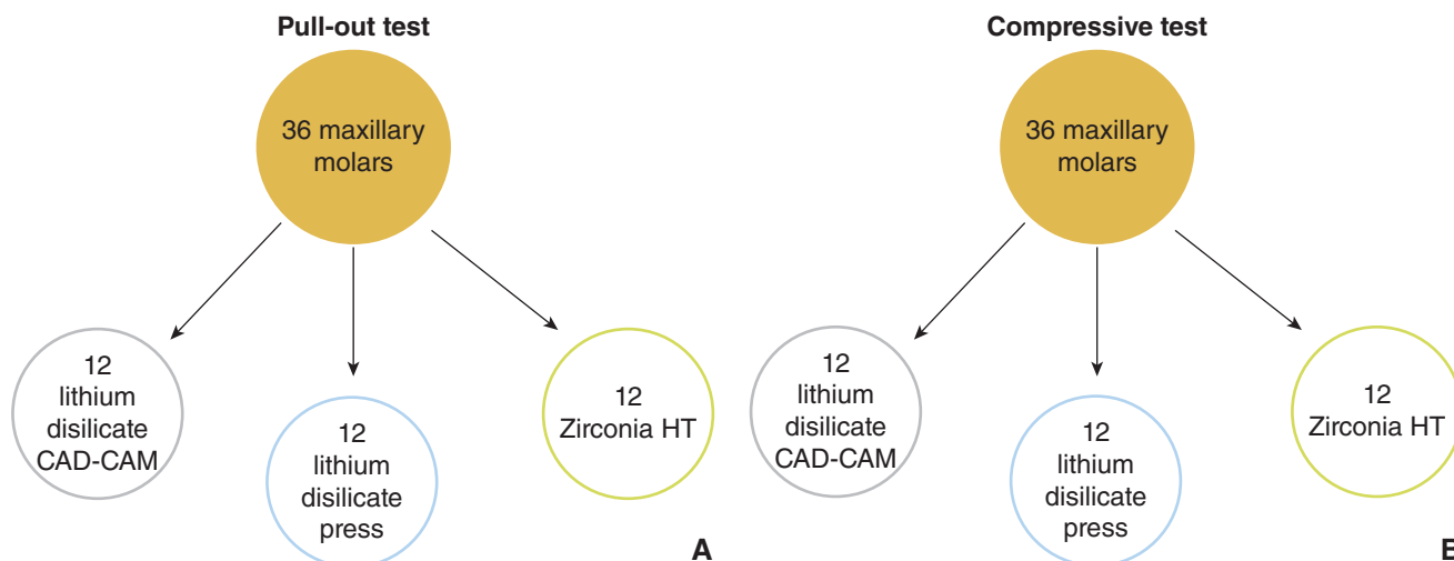
Figure 1. Specimen preparation. A, Pull-out test. B, Compressive test.
