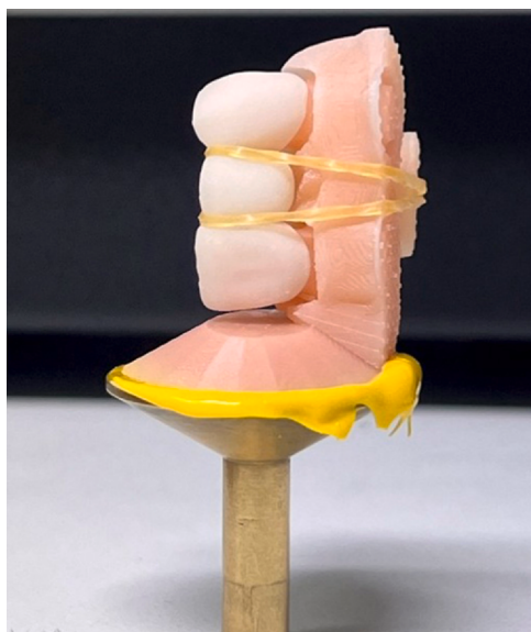
Figure 4. Fixing FDP to cast using elastics and securing assembly to \mu CT tray holder using light-body impression material, FDP, fixed dental prosthesis; \mu CT, microcomputed tomography.
