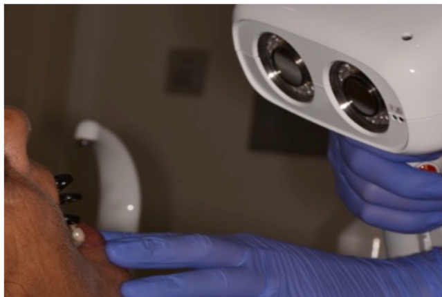
Figure 2. Clinical scenario for recording digital 3-dimensional position of specific stereophotogrammetry scan bodies.
