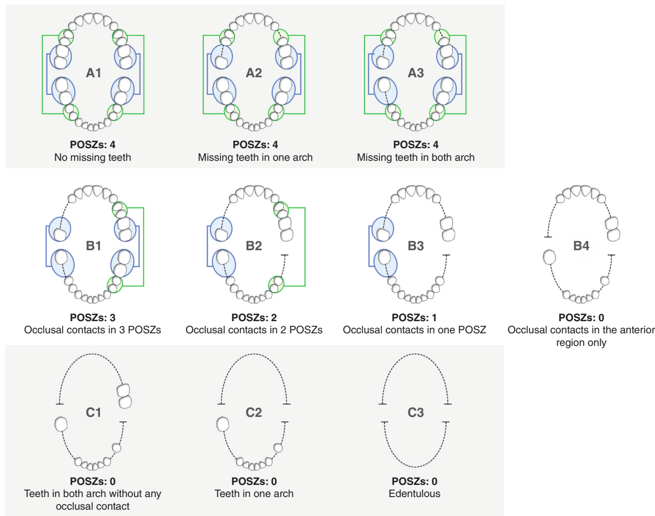
Figure 1. Eichner index and schematic representation. Eichner index evaluates antagonistic occlusal contacts in premolar and molar regions as posterior occlusal support zones (POSZs), indicated by pairs of shaded circles. These regions classified into 4 POSZs, with occlusal support status assessed based on contact within each zone.
